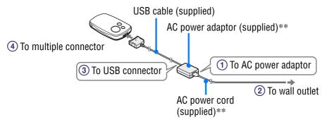
Charging requires the times listed below. When charging finishes, ——lights up on the player, and the light on the USB cable turns off.
